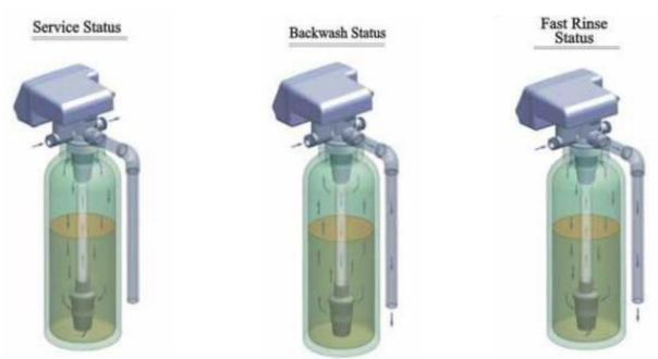
Service Status: Unfiltered water is directed through the media bed and up through the distributor and riser pipe.
