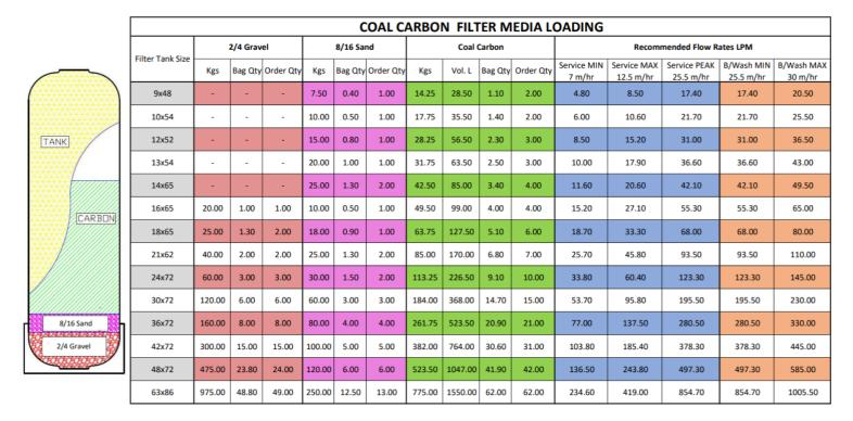
Service & Backwash Flow Rates shown are based on general recommended rates for normal conditions as per Carbon Activated's brochure.
