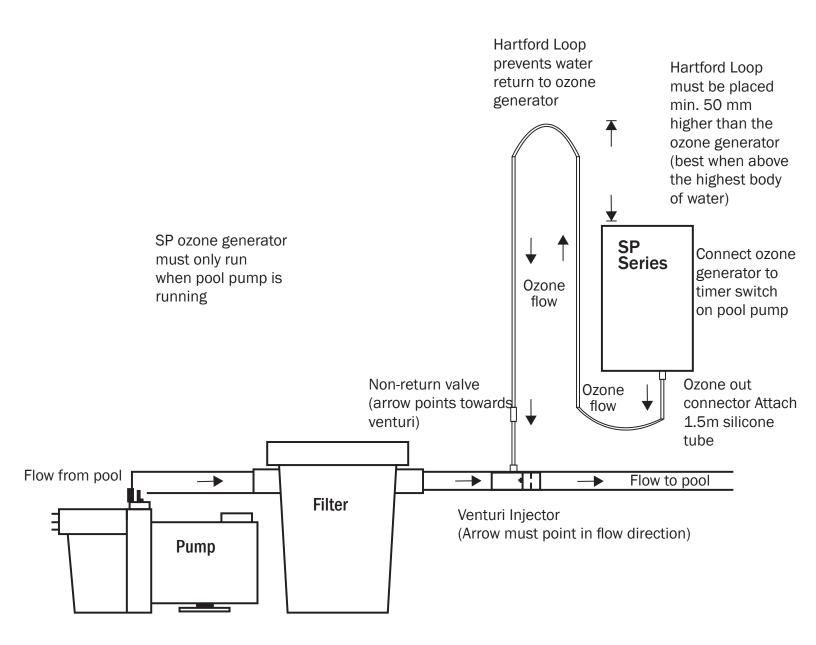
Injector Manifold Point of Installation with "Hartford Loop"
