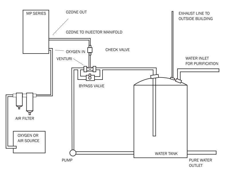
**NOTE:** Ozone generator and ozone line should be above the water tank level. This would prevent of back flow of water to ozone generator.
