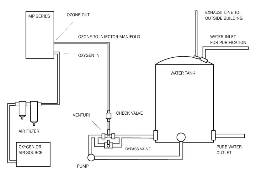
**NOTE:** Ozone generator and ozone line should be above the water tank level. This would prevent of back flow of water to ozone generator.
