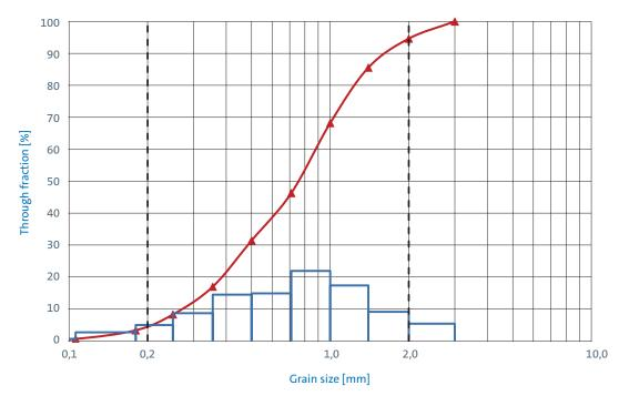
Method of analysis: In accordance with DIN EN 12902 using wet sieving
